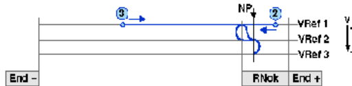
Figure 4.65 Homing mode type 6: The reference cam is flush to the positive hardware limit switch; the first zero pulse after reaching the cam in positive direction is evaluated see Table 4.33
