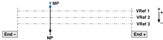
Figure 4.45 Homing mode type 0. The current actual position is set as the reference point. No homing run is carried out. Example: Conveyor belt.
