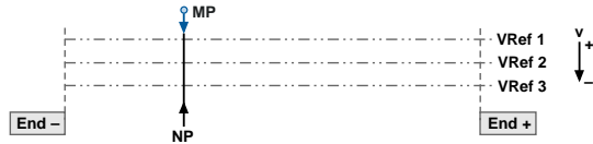
Figure 4.34 Homing mode type 0. The current actual position is set as the reference point. No homing run is carried out. Example: Conveyor belt.
